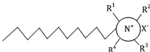
Fig. 7.2: General schematic representation of the structure of a cationic surfactant (quaternary ammonium compounds) ◀
